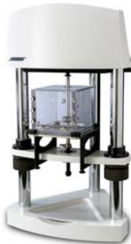
3200 Test Instrument with Saline Bath
