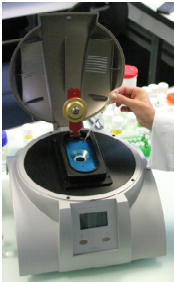
Figure 7 Picture of the “Vasco” instrument and its sample cell
