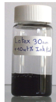
Figure 4 Picture of the latex dispersion after ink addition.
