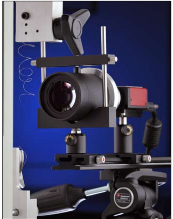
Figure 3. Model LESC Video Extensometer measuring the strain of thin wire.
