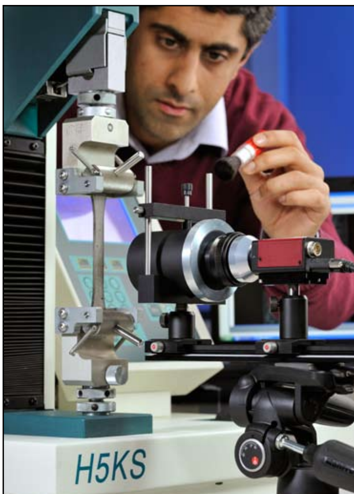
Figure 1. Model H5KS Video Extensometer measuring strain on a plastic specimen.
